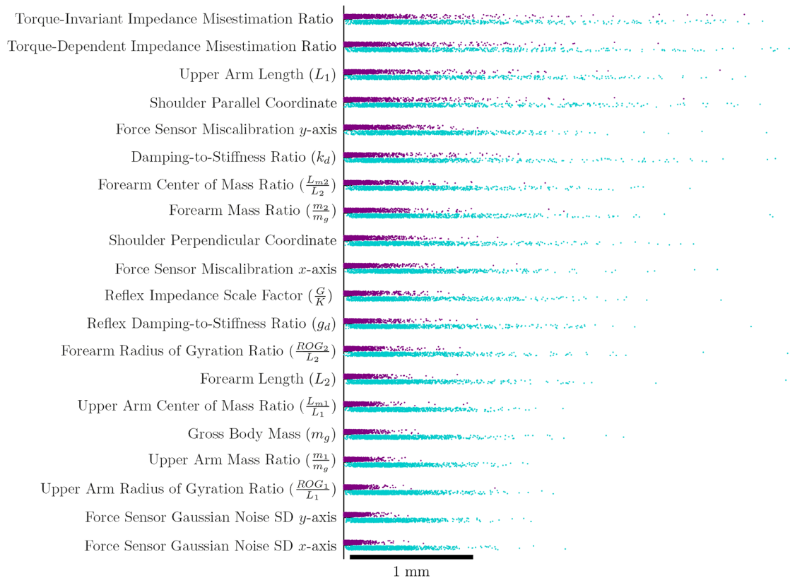
Fig 2. Model sensitivity testing (from the variance-based method of Saltelli et al. [11]) reveals that the model is mostly sensitive to stiffness. Parameter values are varied in a Sobol-distributed fashion according to Table 1. First order sensitivity, in purple, is the error that would be removed if the parameter was fixed at its nominal value. Total sensitivity, in teal, shows error that would remain if all other parameters were fixed at their nominal values.
