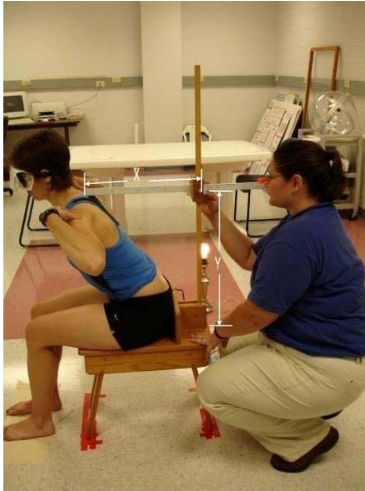
Figure 4 The measurement method: The X and Y coordinates are shown above with an individual in a position 2/3 of full flexion; during the study, all subjects were blindfolded throughout testing.
