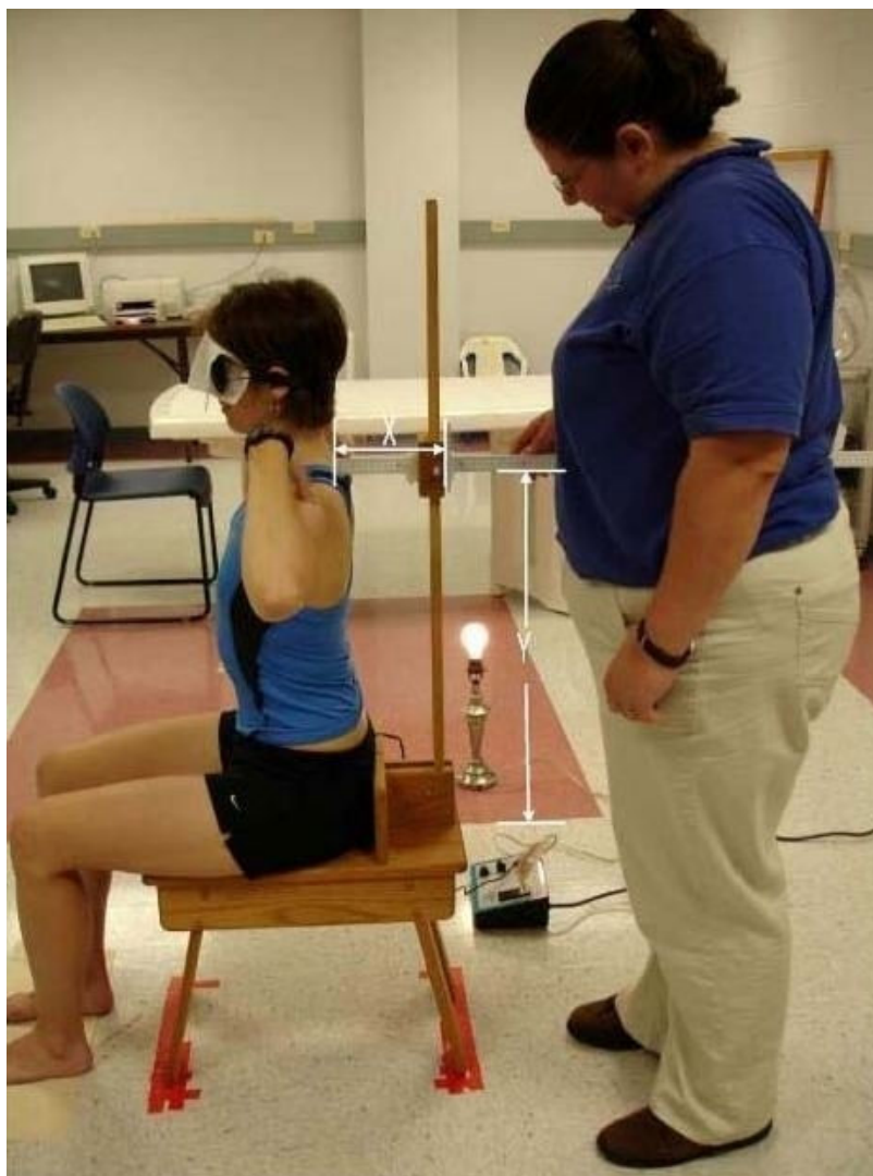
Figure 1 The measurement method: X and Y coordinates are measured and used in a trigonometric calculation to determine the angle. An individual is shown seated in the upright neutral posture; during the study, all subjects were blindfolded throughout testing.
