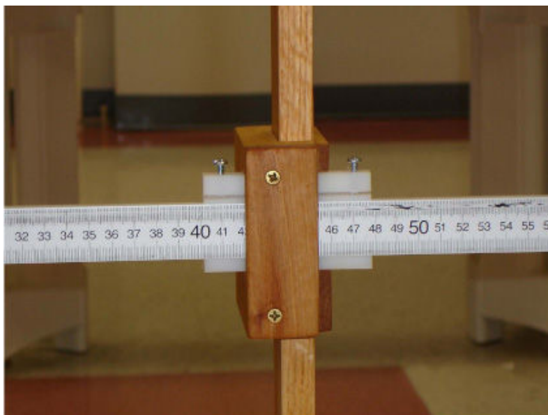
Figure 3 Horizontal measurement view for the new SRSD method taken from the side of the sliding mechanism.
