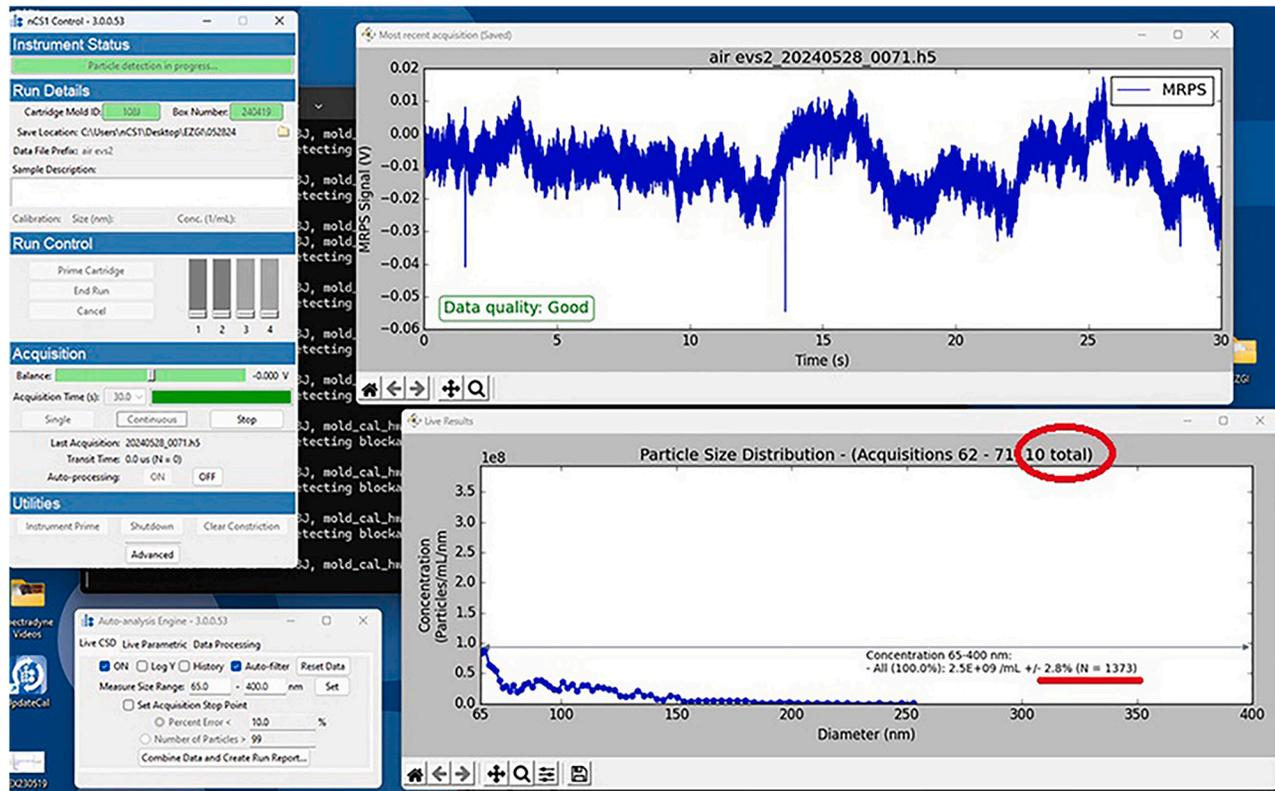
**Figure 7. Screenshot of the Spectradyne software demonstrating the EV concentration readout with a minimum of 10 total reads and accurate reading percentage of  $\pm 2\%$**
