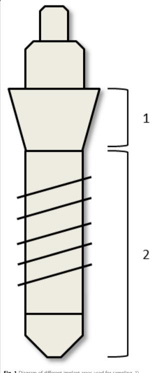
**Fig. 1** Diagram of different implant areas used for sampling. 1) Machined (untreated) area. 2) rough (treated) area
