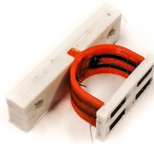
**Figure 7.** Photograph of the printed sensor with the strain gauges positioned on the inside. The conductive TPU parts are shown in black, non-conductive TPU in orange, and the PETG parts in white.
