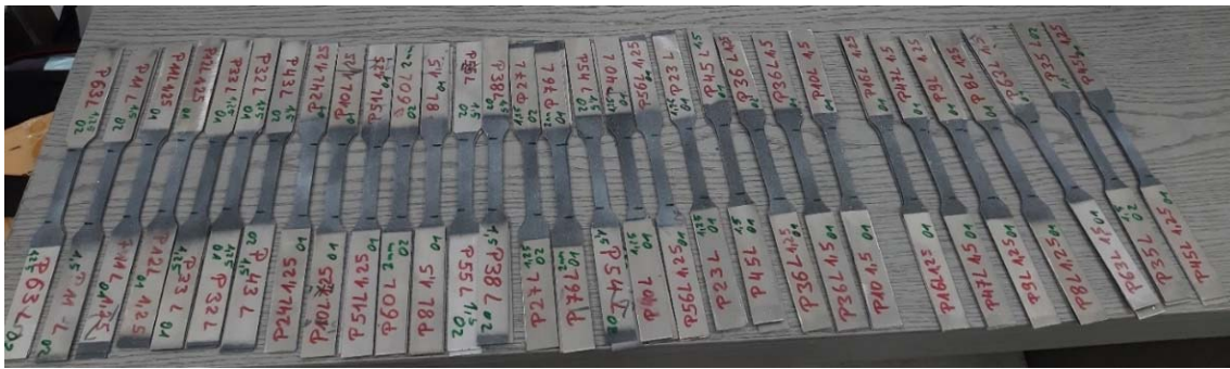
Figure 2. A photo of specimens prepared for the static tensile test with the use of a digital image correlation system (DIC).
