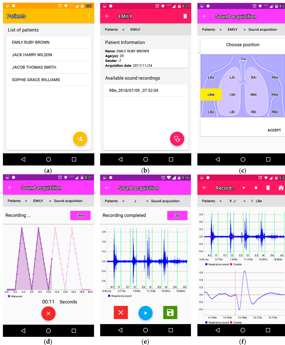
Figure 7. Different activities of the mobile app. (a) Patient list activity. (b) Patient activity. (c) Selection of auscultation point activity. (d) Sound recording activity. The area under the curve fills during the acquisition to provide a visual aid. (e) Activity to replay, discard or save the recording. (f) Analyze patient activity. The upper graph displays the whole recorded respiratory sound and the detected locations of crackles. This graph is fixed. The bottom graph displays a segment of the signal selected by the user so that it can be zoomed, scrolled and tactile select a data point to know its exact time location on the screen.
