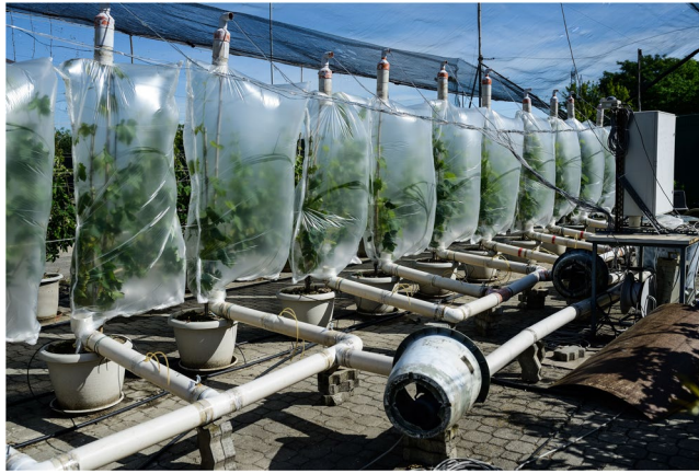
Figure 1. General view of the whole-canopy gas exchange system set up at the beginning of measurements.
