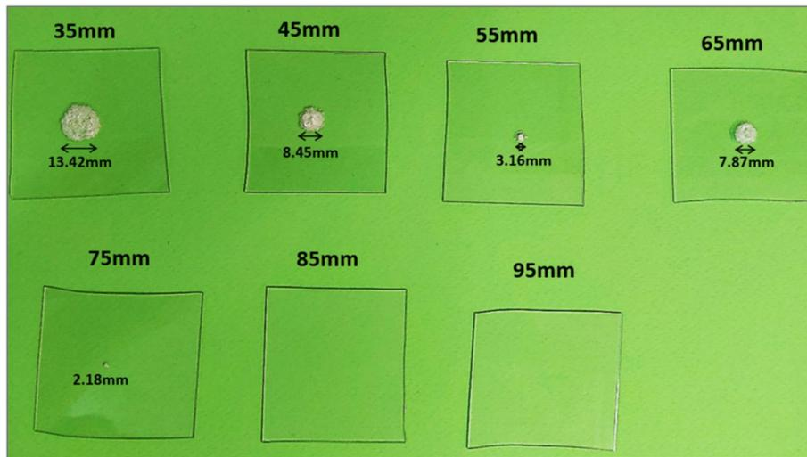
**FIGURE 6** Photo of films sonicated at increasing depth from the surface of a single element transducer with central frequency of 2.75 MHz, radius of curvature of 65 mm, and diameter of 50 mm, indicating the diameter of the formed lesions
