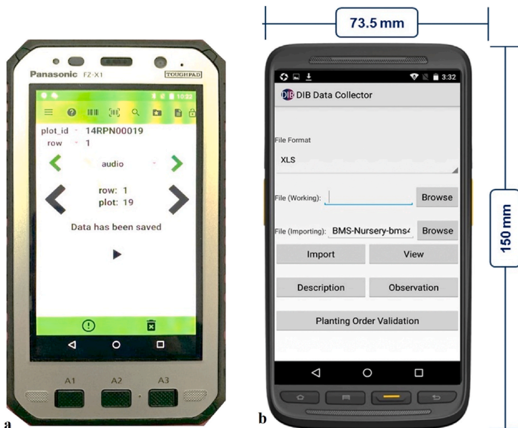
Fig. 1. Handheld devices for data recording a) Panasonic toughpad b) Digital data collector.
