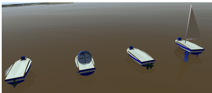
Figure 4. From left to right: the rudder boat, airboat, differential boat and sailboat available in the simulator.
