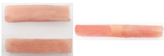
Figure 1a Specimens ready for hardness test b Specimens ready for tensile test
