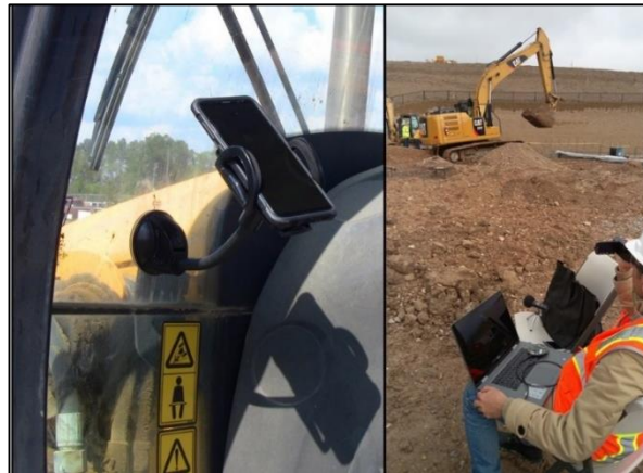
Figure 11. Configuration of audio and kinematic recording devices in a sample job site.
