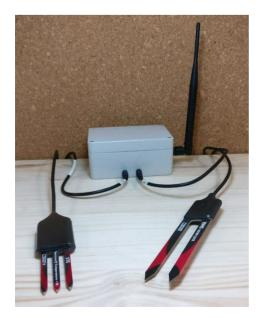
Figure 4. Node with ECH2O soil moisture sensors.
