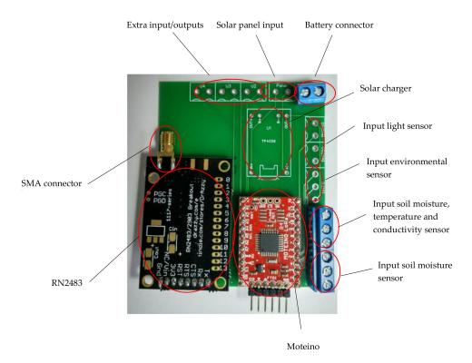
Figure 1. Photograph of the wireless sensor node.
