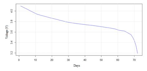
Figure 5. Node battery voltage.
