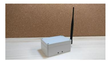
Figure 2. Node sensor (end-device for the lab test).
