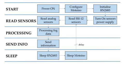
Figure 3. Flow chart of the node sensors.
