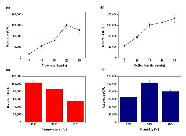
**Figure 3.** Investigation of various variables for airborne bacteria collection kit. All CFU values were measured by qPCR curves, N = 3. (a) Flow rate of air pump testing, (b) bacteria collection results for pump operation time, (c) bacteria collection results by different temperatures, and (d) collection results by humidity.
