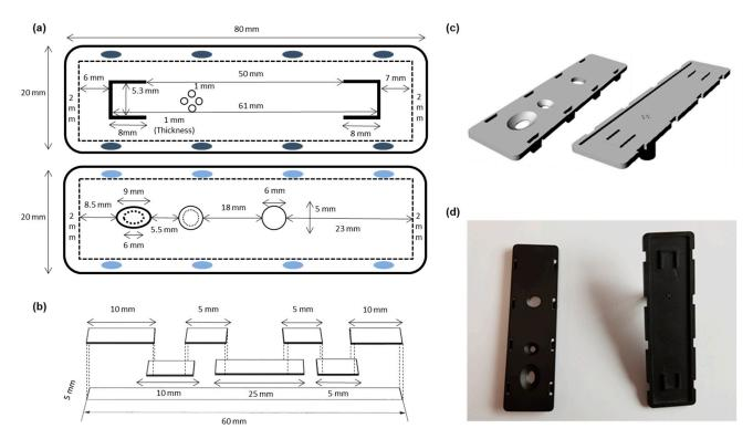
**Figure 2.** 3D printing of airborne bacteria collection kit. (**a**) Hand drawing of the 3D printing chip, (**b**) simple drawing of the paper strip with assembly line in the case, (**c**) CAD image, and (**d**) photograph of printed case.
