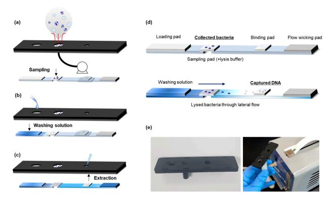
**Figure 1.** Workflow of the paper kit: (**a**) aerosol sample collection using air pump, (**b**) loading of washing solution at hole in the case, (**c**) DNA extraction through lateral flow in the strip, (**d**) schematic of aerosol collection and DNA extraction process, and (**e**) photographs of the paper kit with 3D-printed case and air pump.
