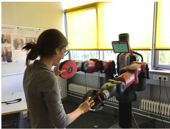
Fig. 1 Example human-robot exercise game interaction. Our customization of this robot's facial expressions and end-effectors help Baxter serve as a gameplay partner
