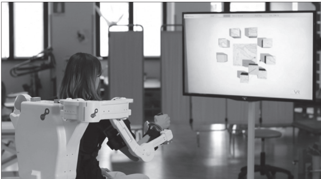
Figure 1. The Alex 2 exoskeleton developed by Scuola Sant'Anna (commercialized by Wearable Robotics srl) integrated with a serious rehabilitation game.
