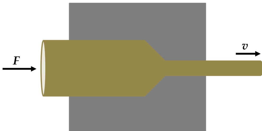
Figure 1. Schematic diagram of the extrusion process.
