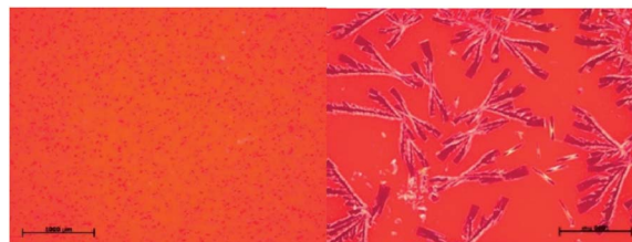
Fig. 6 Microscopic images of Shin(1)LG305 2000 ppm (100 \times optical magnification). After the curing process (150 °C, 4 h) small crystallites were detected (left). An additional heat treatment of the cured sample (200 °C, 120 h) resulted in a crystal growth in the cured, solid matrix.
