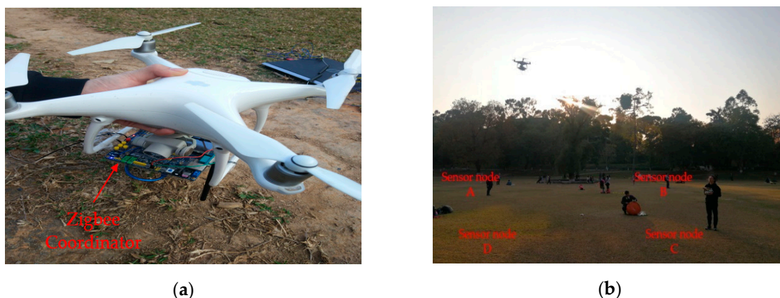
Figure 14. Communication test between UAV and ground WSN nodes. (a) UAV with Zigbee Coordinator; (b) Ground wireless sensor nodes.
