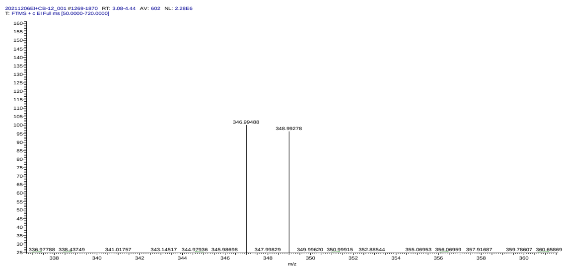
Supplementary Fig 35. EI mass spectrum of R -4FBrBI.
