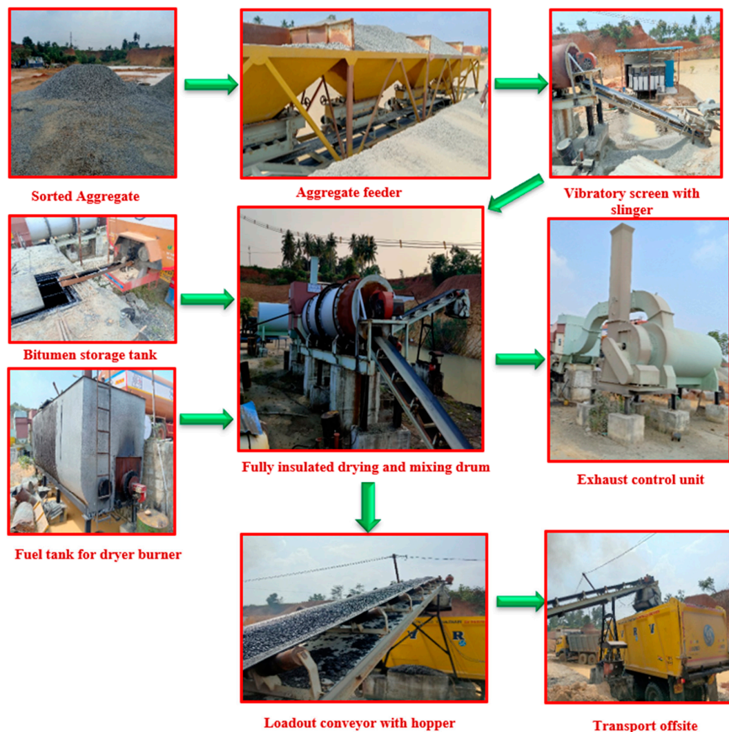
Figure 5. Preparation and production of coarse aggregate coated with asphalt.
