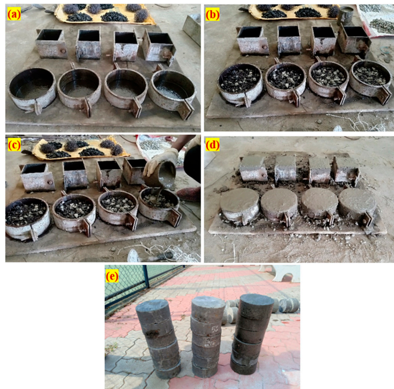
Figure 6. PAFC casting procedure (a) empty mold, (b) fibres and aggregates are filled in the mold, (c) grouting under gravity, (d) finished specimens and (e) specimens after demolding.
