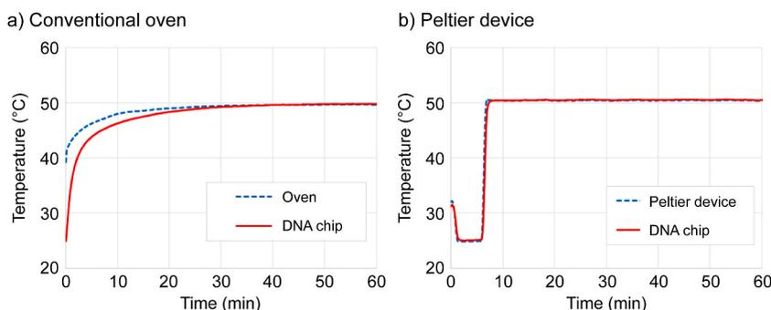
Fig. 2. Comparison of heating time between (A) conventional oven and (B) our DNA microarray system using a Peltier device.
