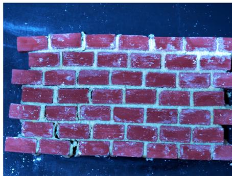
**Figure 1.** A sample image of wall built and cracked in the lab.
