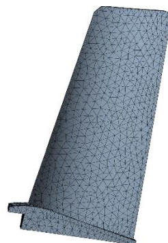
Figure 3. Finite element model of the blade.
