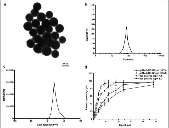
Fig. 1 Characterization of Gefitinib/CQ-NPs, **a** TEM images of Gefitinib/CQ-NPs, **b** DLS analysis of Gefitinib/CQ-NPs, **c** zeta potential of Gefitinib/CQ-NPs, and **d** accumulative release of Gefitinib/CQ-NPs and free Gefitinib in the medium at different pH. The results were expressed as mean  $\pm$  SD (n = 3)
