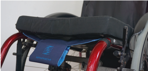
Fig. 1 Textile pressure system. Textile pressure mat of the feedback system (placed underneath the skin protection wheelchair cushion) with the data acquisition/transmission unit (located in the small flap with the company logo).
