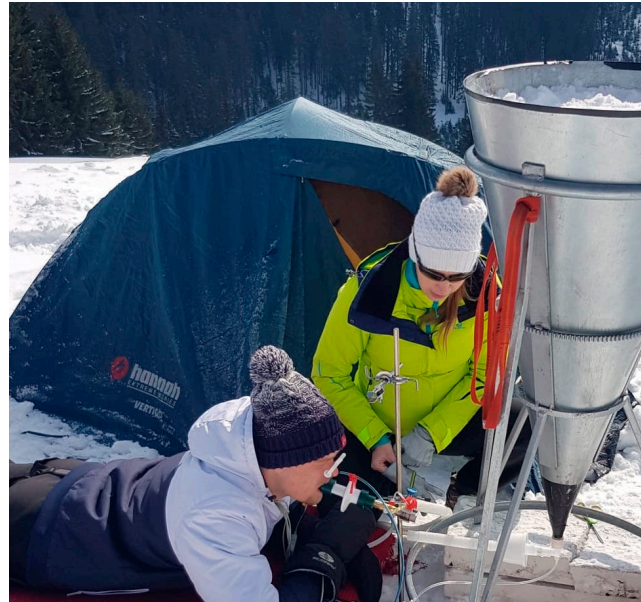
Figure 2. A photo from the stabilization phase of the experiment. Subject is in a prone position, lying on an insulated mat, breathing through a mouthpiece connected to a monitor. The specially designed tubing is ready to be connected to the cone-shaped container filled with material simulating avalanche snow. The subject is monitored closely by the attending physician.
