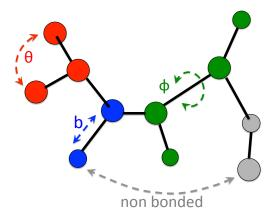
**Figure 4.** Typical interactions considered in a all-atomistic force field. Atoms of a molecules interact by simple springs, in lengths and angles (bonded contributions), and via long range forces (non bonded contributions). In a mechanical view the forces determine the spatial arrangements of atoms an their dynamics.
