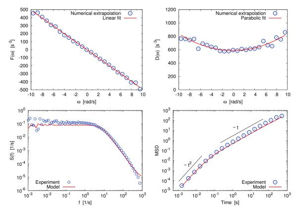
**Figure 6.** Dilute granular experiment. Top: Reconstructed drift (**left**) and diffusivity (**right**) for the angular velocity, fitted trough a linear function and a quadratic polynomial, respectively. Bottom: Power spectrum (**left**) and mean square displacement (**right**); experimental data (blue circles) are compared to those obtained by simulating the inferred stochastic model (red lines).
