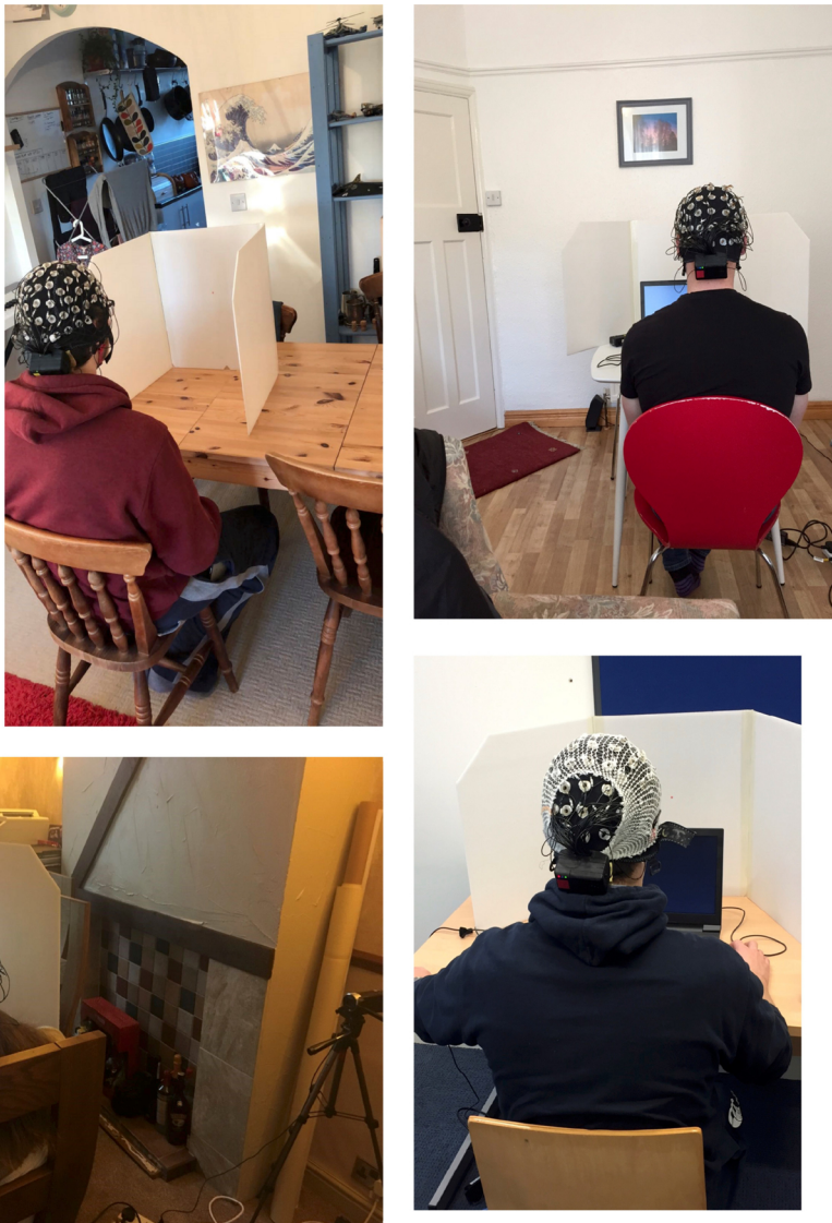
Fig. 6. Illustration of large-scale mobile EEG testing across indoor locations using conventional stimuli presentation. Photographs were taken as part of regular research documentation to fine-tune testing protocol and inform standardization. Four mobile set-ups using a mobile EEG headset from Cognionics in clockwise order: testing in a home setting and of resting state recordings, which include folding panels to reduce visual distraction, having participants' backs facing the window to reduce visual interference and having the researcher out-of-sight to allow for minimal interference and note-taking; testing also in a home setting with a similar set-up, this time of a task-based paradigm using stimuli delivery via a laptop; testing in an office setting, illustrating the use of a soft cotton-net to reduce cable movement if required; finally, testing in a home setting, with camera positioned to allow for recording of potential full-body movements/facial expressions for later revisions.
