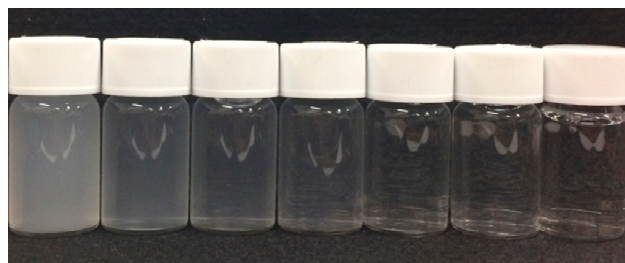
Figure 4. The 7 different concentration calibration solutions of kaolin: From left to right, the concentrations are 500, 200, 100, 50, 20, 10, and 0 mg/L.
