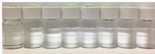
Figure 12. The 8 different concentration calibration solutions of chlorophyll a : From left to right, the concentrations are 500, 200, 100, 50, 20, 10, 5, and 0 \mu\text{g/L} .
