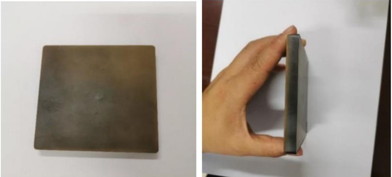
Figure 4. The B 4 C/TiO 2 /polyimide molded plate.
