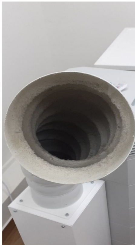
Figure 5. Hose contaminated from microparticles (School of Dentistry, National and Kapodistrian University of Athens).
