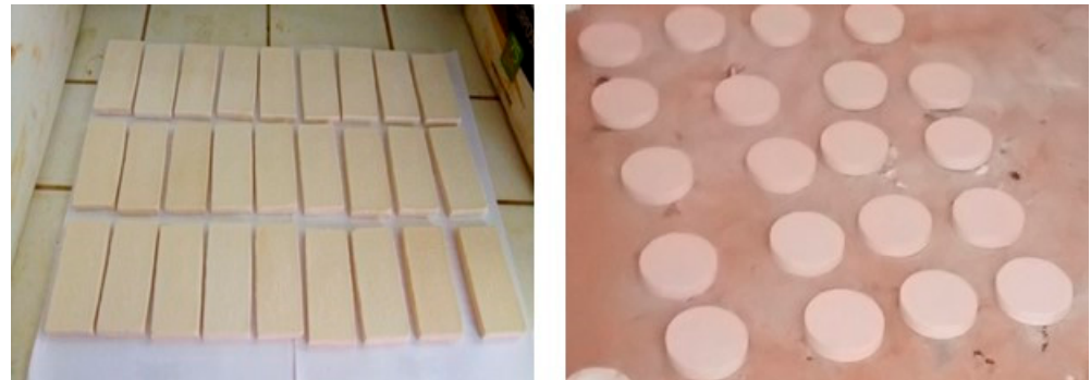
Figure 4. Physical aspect of membranes after sintering at 1150 °C.
