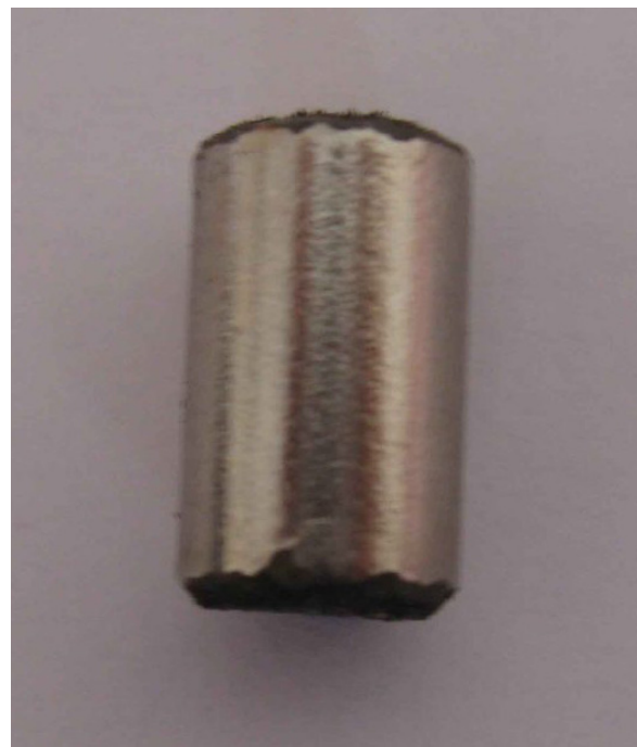
Figure 3. Cobalt samarium magnet used to combine the prostheses.
