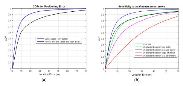
Figure 7. (a) Localisation performance for the two environments. (b) Sensitivity to measurement errors.
