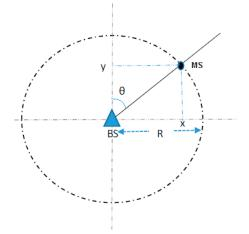
Figure 4. Obtaining the second coordinate for LOS scenarios [3].
