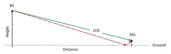
Figure 3. Ground reflected multipath (red dashed path).
