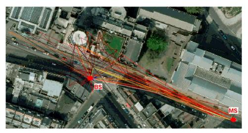
Figure 1. Multipath rays for a BS-MS point-to-point link.
