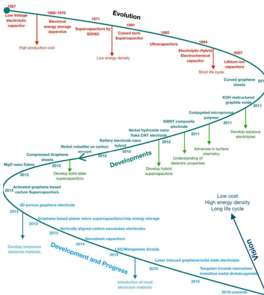
Figure 13. Roadmap of the evolution, progress, and developments of supercapacitors. Reproduced with permission from [126].
