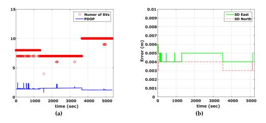
**Figure 8.** Number of visible satellites and PDOP values for the vehicle maneuvering test (**a**), and estimated position standard deviation (**b**).
