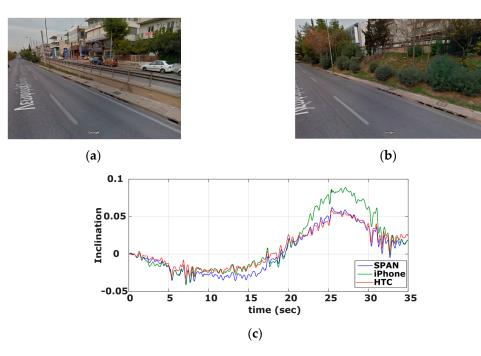
**Figure 20.** Vertical profile of exit ramp computed using smartphone gyroscopes. Ramp elevation at entrance (**a**) and exit points (**b**), and computed road inclination (**c**).
