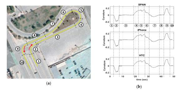
**Figure 19.** Road curvature compution using smartphone IMUs. Travelled trajectory (**a**), and extracted road curvature diagrams (**b**).
