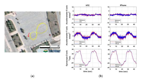
**Figure 16.** The Figure 8-shaped special maneuver. Travelled trajectory (**a**), and smartphone IMU sensor readings (**b**).
