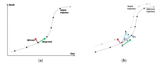
**Figure 2.** Along-/off-track coordinate system (i.e., body frame) (**a**), and observation geometry involved in positioning trueness definition of a moving vehicle (**b**).
