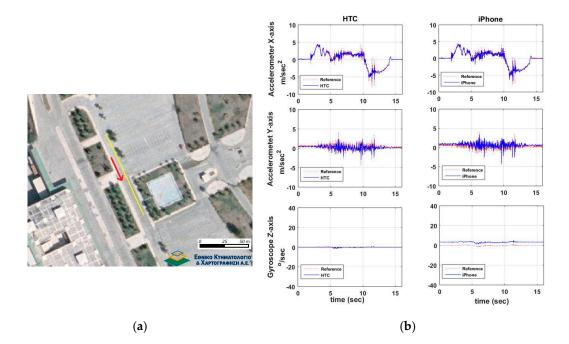
**Figure 12.** A typical speeding-stopping maneuver that consists of an aggressive acceleration and deceleration part on a straight line path. Travelled trajectory (**a**) and smartphone IMU sensor readings (**b**).
