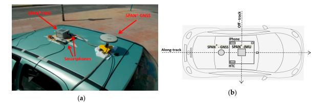
Figure 3. Navigation sensors mounted on top of the test vehicle.
