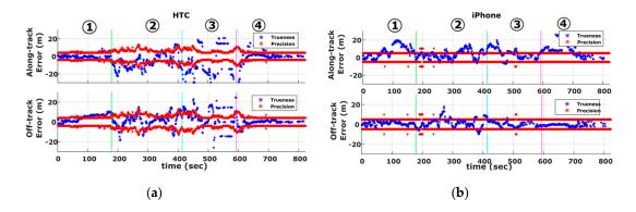
**Figure 9.** Along-track and off-track GNSS trueness and precision measures obtained for the HTC One S (**a**) and iPhone 5s (**b**) during the cruising scenario.
