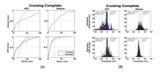
**Figure 10.** CDF-Cumulative distribution functions (**a**), and probability density histograms (**b**) of the GNSS trueness and precision measures obtained for the complete run of the cruising tests.
