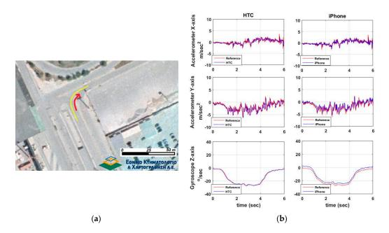
**Figure 14.** A typical turning maneuver of a 90° right turn. Travelled trajectory (**a**), and smartphone IMU sensors readings (**b**).
