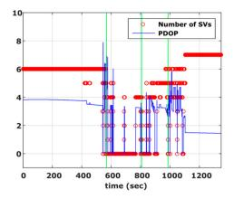
**Figure 5.** Cruising scenario. Number of visible satellites and PDOP values obtained for the complete travel path. The vertical lines represent the start/end of the deep urban and tree covered sections respectively.
