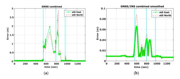
**Figure 6.** Estimated standard deviation for the GPS-only navigation solution (**a**), and for the smoothed/combined GPS/IMU navigation solution (**b**).
