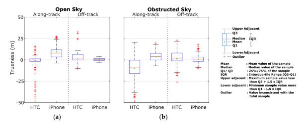
**Figure 18.** Box and whiskers plot obtained for the GNSS trueness for the open sky (**a**), and obstructed sky conditions (**b**) considering the complete test series of the vehicle cruising trials.
