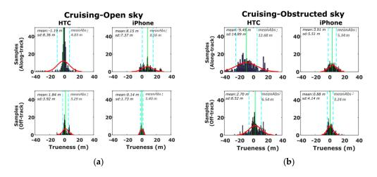
**Figure 11.** Probability density histograms of the along- and off-track smartphone GNSS trueness for the open-sky (**a**), and obstructed-sky (**b**) sections of the cruising scenario.
