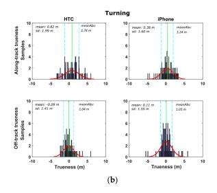
**Figure 15.** Probability density distributions obtained for the smartphone trueness for the IMU (**a**), and GNSS (**b**) readings considering the complete set of the turning tests.
