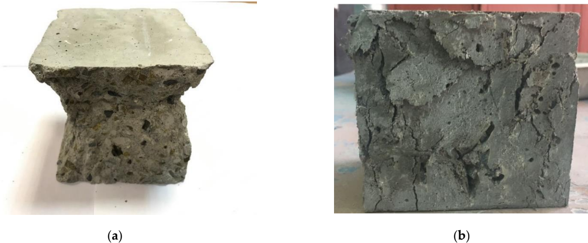
Figure 7. The nature of the destruction of samples of (a) concrete without fibers; (b) fiber concrete.
