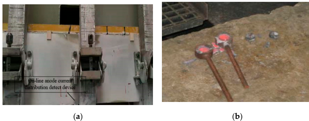
Figure 9. In situ data collection: (a) online collection of anode current distribution in aluminum reduction cell; (b) alumina concentration sampling for inspection.
