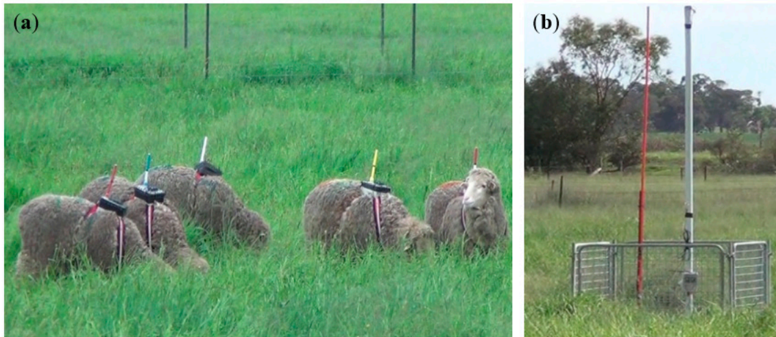
Figure 4. RTK rovers fitted on the back of sheep via harnesses (a), and fixed base station (b) in the middle of the paddock. The two masts (b) were for the GNSS amplified antenna, and RTK correction transmitter.
