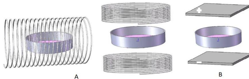
**Figure 4.** Two designs offering noninvasive ES. (A) ES through EMF, where a cell culture plate is placed inside a Helmholtz coil in parallel to the direction of MF, or in perpendicular to the direction of MF between two Helmholtz coils; (B) ES through capacitive coupling where a culture plate is sandwiched between two parallel plates (note: the distance between plates and culture should be minimum to reduce resistance).
