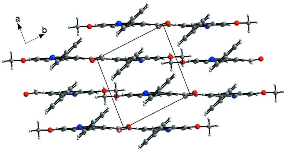
**Figure 2**(Brandenburg & Berndt, 2001) A alternating layers parallel to (210)planes of (I) viewed down the *c* axis.
