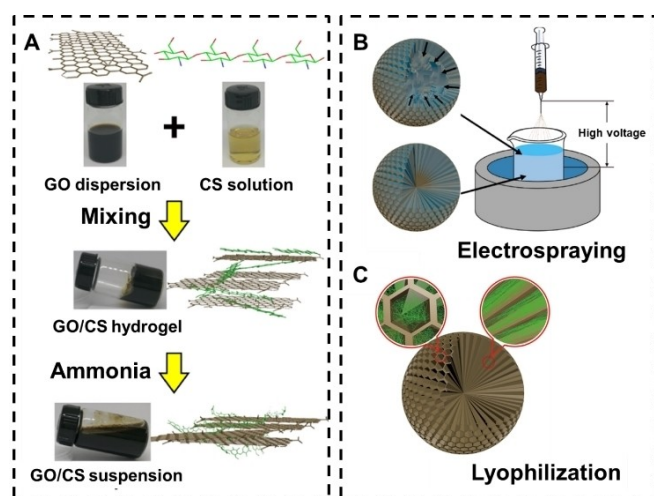
Figure 5. Preparation scheme of GO/CS microspheres. Reproduced from Yu et al., [66] Copyright 2017, with permission of the American Chemical Society.
