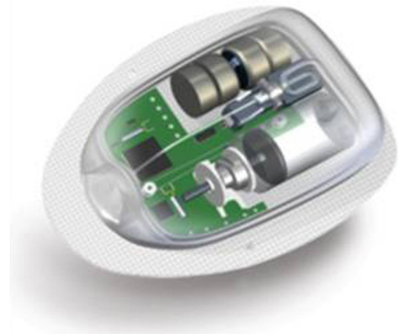
Figure 3. A look under the hood, featuring core components of the OnmiPod.
