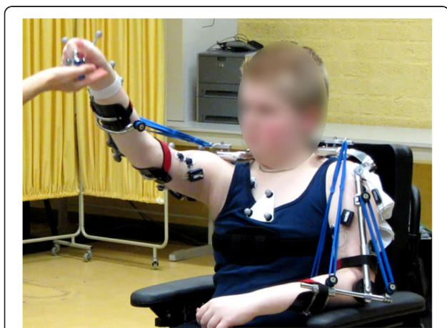
Fig. 4 Boy with Duchenne testing the prototype, while wearing electromyography and motion capturing devices
