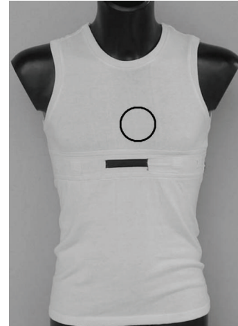
FIGURE 2: Prototype of the inner garment in which the wearable wireless interface for the detection of the heart and breath rates will be included. In detail, the sensor will be placed around the circled area.
