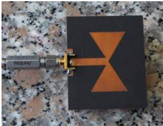
FIGURE 10: Antenna prototype for the channel model verification.
