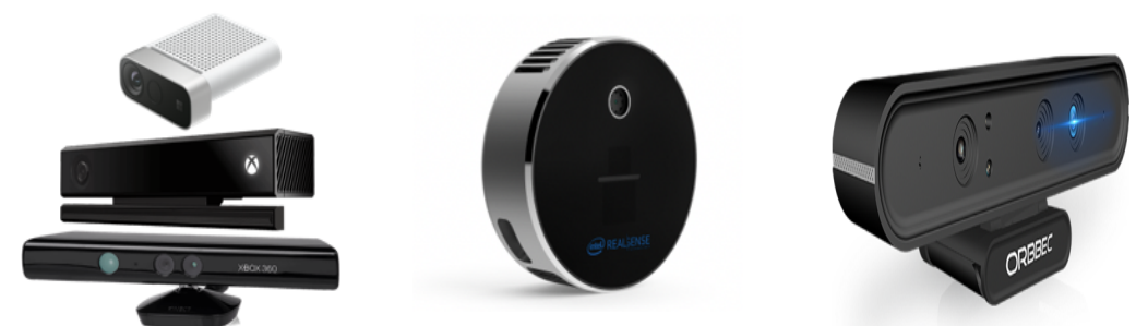
Figure 3. Various RGB-D sensors: (a) Microsoft Kinect [33–35], (b) Intel RealSense L515 [36], and (c) Orbbec Astra Pro [37].
