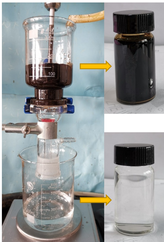
Figure 6. Separation of asphalt-containing oil–water mixtures with CECS aerogels.
