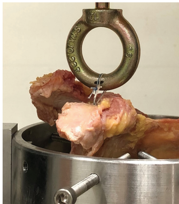
Figure 1. The biomechanical setup. Each specimen was mounted on a universal materials testing system. The suture ends of the anchors were tied together on the adapter of the materials testing machine. The distance between the inferior border of the adapter and superior cortex of the coracoid bone was standardized: 10 mm in the superior-inferior direction and 6 mm in the anterior-posterior direction, resulting in a spatial distance of 12 mm.
